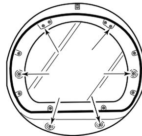
5. Lift the inner door assembly off of the outer door assembly. Set the outer door assembly aside.
