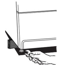
If the dryer is not level, prop up the dryer using a wood block. Use a wrench to adjust the legs up or down and check again for levelness.
