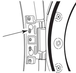
2. Lift and pull forward on the door so that the screwhead clears the keyhole. Remove the door.
