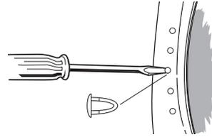
6. Insert a screw in the second opening from the top of the hinge opening and partially tighten. Hang the door by placing the top hinge keyhole over the second screwhead and tighten the screw. By putting this screw in first, the door will hang in place while you insert and tighten the remaining 4 screws.
