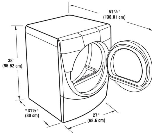
\* Most installations require a minimum 5 1/2 in. (14 cm) clearance behind the dryer for the exhaust vent with elbow. See "Venting Requirements."
