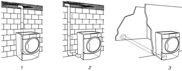
1. Standard rear offset exhaust installation
