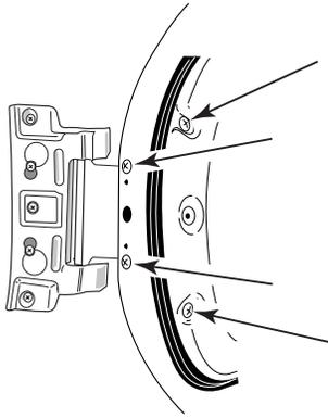
3. Remove the 2 screws that hold the handle bracket to the door.
